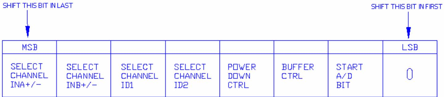
**Figure 3: GyroPoint ASIC Input Control Word**
