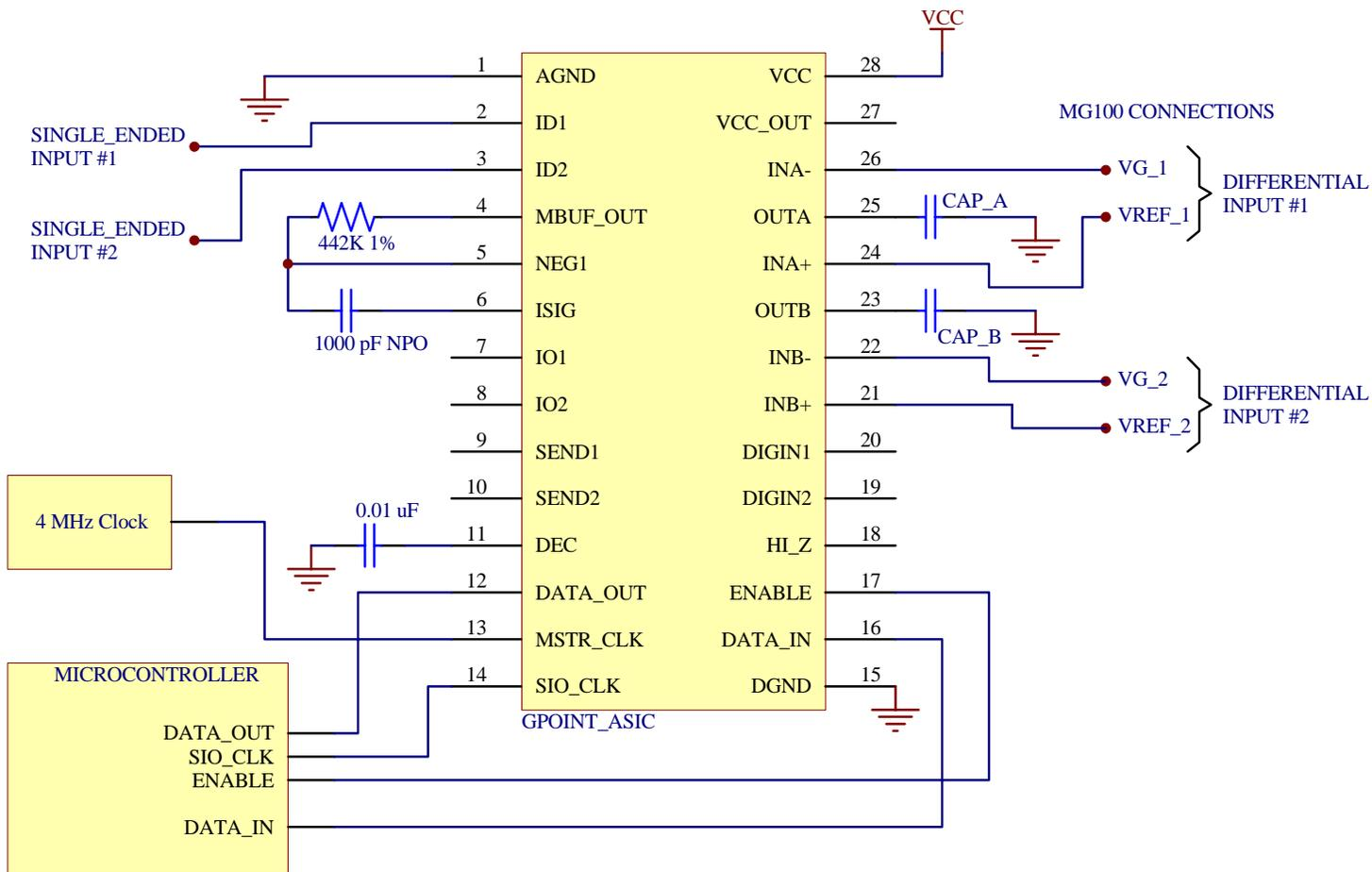
**Figure 1: GyroPoint ASIC Hookup Diagram**
