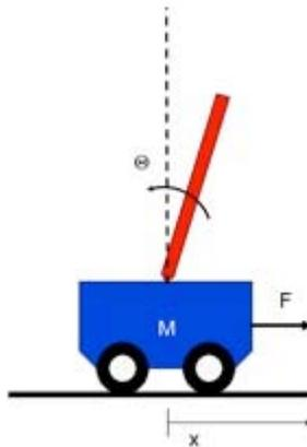
In this image, the cart is the Blue object and the pole is the Red object. The lowest point on the pole is where the pole and cart are attached through a mechanical device that allows the pole to rotate.
