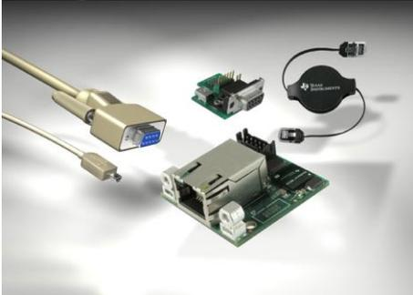
The Stellaris RDK-S2E device implements a telnet networking server and a TTL Serial UART interface. We connected the Ethernet interface to the WiFi router and the TTL Serial UART Serial interface to the ATXMEGA 128 8-bit microprocessor. With this configuration, the Android application can open a networking connection and can send and receive data from the ATXMEGA128 8-bit microprocessor's UART connection as if it was a network-connected device.
